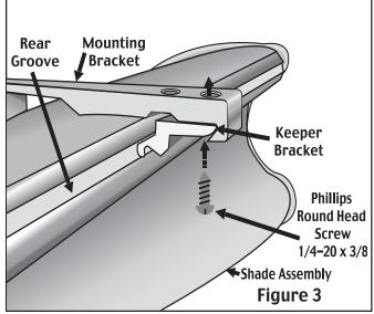
**STEP 5.** Make sure that the slot in the small keeper bracket is aligned with the threaded hole in the mounting bracket. Secure them together using the supplied  $\frac{1}{4}$ -20 x 3/8" Phillips screw. Repeat for the other side. Your installation is complete.
