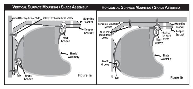
**STEP 1**. Determine the desired location for the mounting brackets, making sure that they are plumb and level. Using a pencil, mark the 2 hole locations in the bracket. Using a 1/8" bit, drill holes approximately 1-1/2" deep at both hole locations. Repeat for the mounting bracket on the other side.
